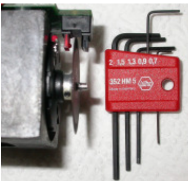
GOOD ENCODER POSITIONING WITH 0.9MM ALLEN KEY
