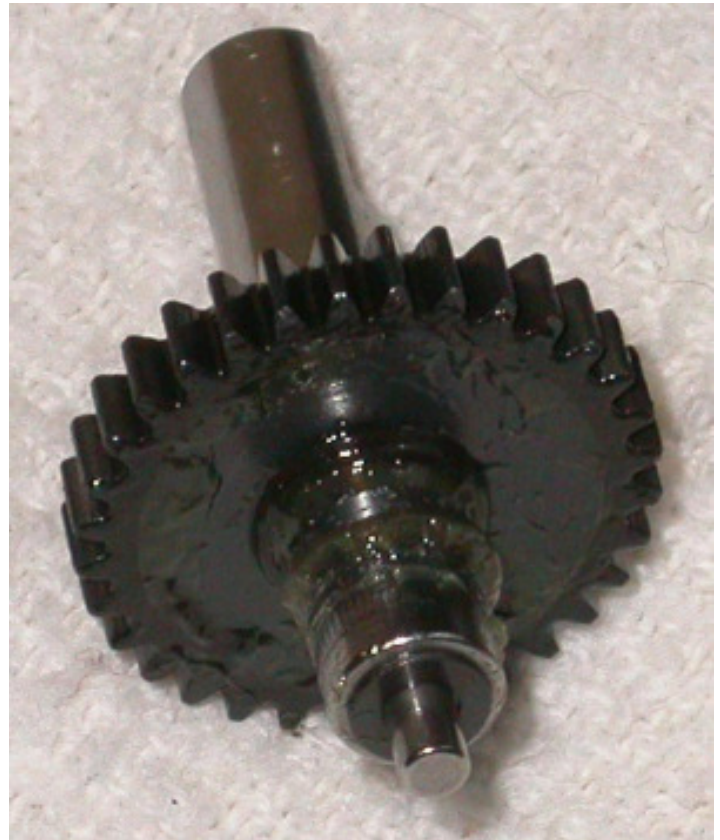
THE MAIN KEYED GEAR AFTER IT IS REMOVED FROM THE HOUSING. BE CAREFUL NOT TO LOOSE THE TWO WASHER-BEARINGS AS PICTURED BELOW.
